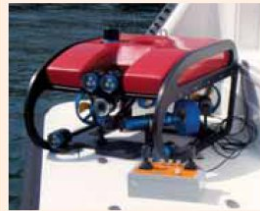
The Pro 4 ROV positions via its Smart Tether, made by KCF Technologies. Photo courtesy of Brett Seymour, National Park Service Submerged Resources Center.
